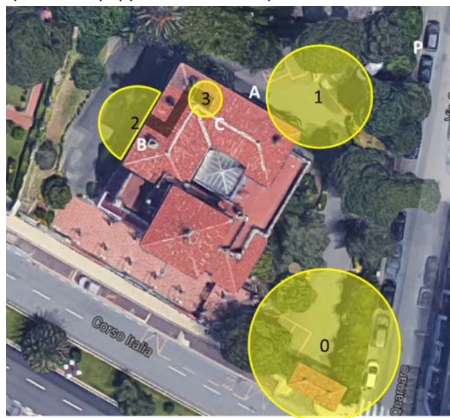
Figure 23. Indicative placement of ABBI Audio Beacons in Chiossone's villa . P: Parking. A: Entrance (not used). B: Entrance. C: Elevator. 0,1,2,3: Target Audio Beacons location
